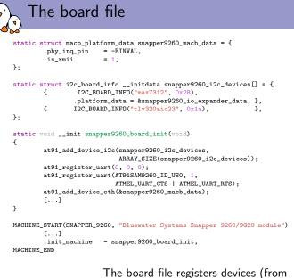
The board file registers devices (from arch/arm/mach-at91/board-snapper9260.c)
